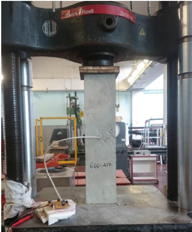
Fig. 6. Test on 16 \times 16 \times 64 cm column
