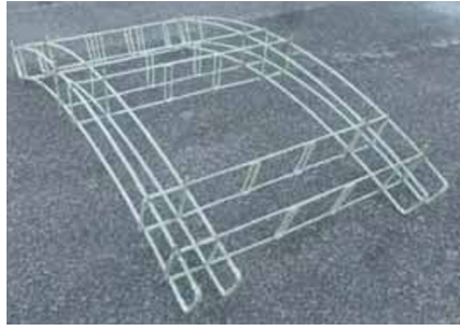
Fig. 2. Perimetric GFRP reinforcement cage.
