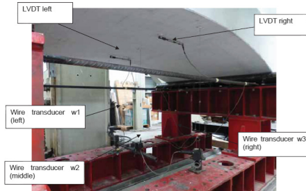
Fig. 8. Bending test instrumentation.
