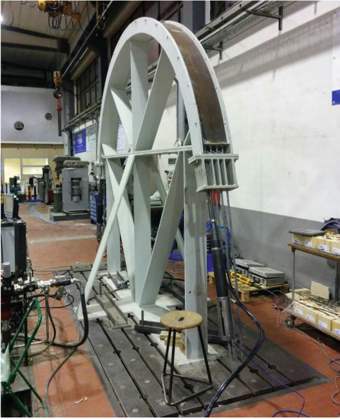
Fig. 5. Friction test carried out over a multi-tube saddle with small radius of curvature.
