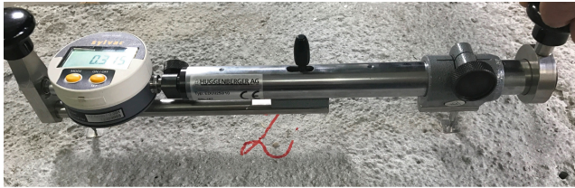
Fig. 2b. Shrinkage measurement
