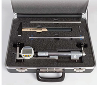
Fig. 2a. Shrinkage measuring instrument (deformeter)
