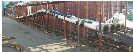
Fig. 8. Picture showing tendons assembled and exposed during the 14 days testing period
