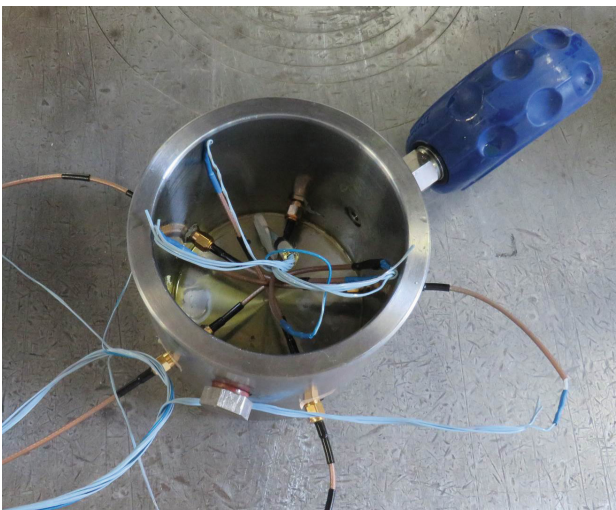
Fig. 4. Hydrostatic load cell for “HYD” test
