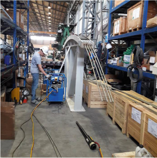
Fig. 4. Friction test carried out over a multi-tube saddle with great radius of curvature (flat saddle)
