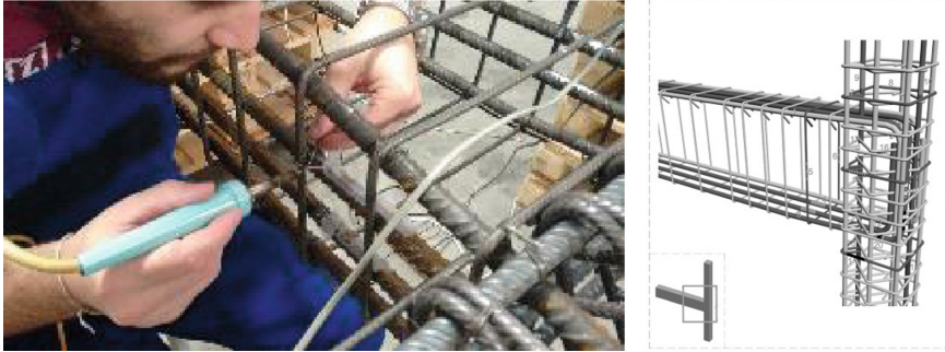
Fig. 6. Strain gages application and disposition
