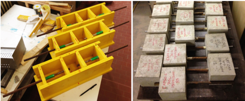
Fig. 1. Pull-out molds and specimens
