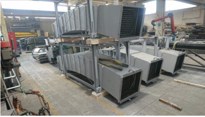
Fig. 1. Multi-tube saddles for 127-strand stay cables stocked in the workshop
